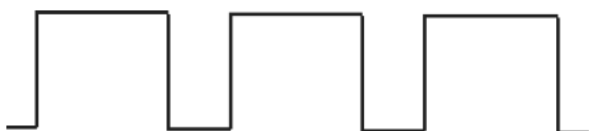
Forward power sensor signal waveforms
