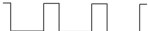
Reverse power sensor signal waveforms
